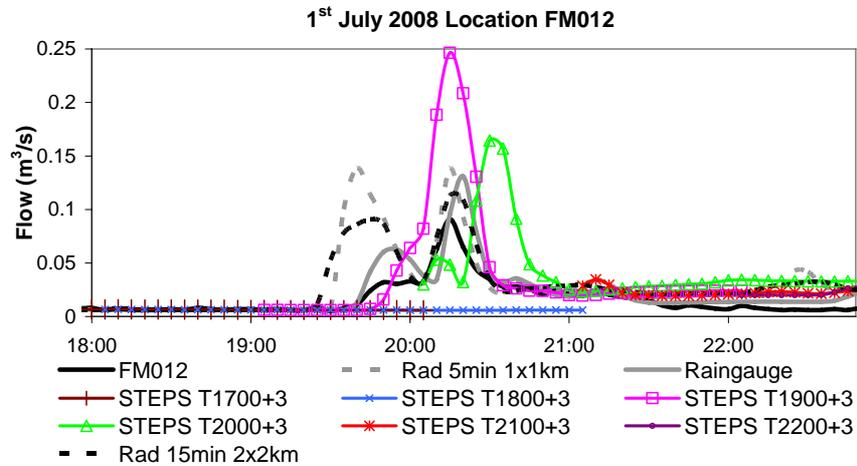
Figure 3 – Sewer flow simulations compared with measured flow, at flow monitor location 012, for the 1<sup>st</sup> of July 2008.
