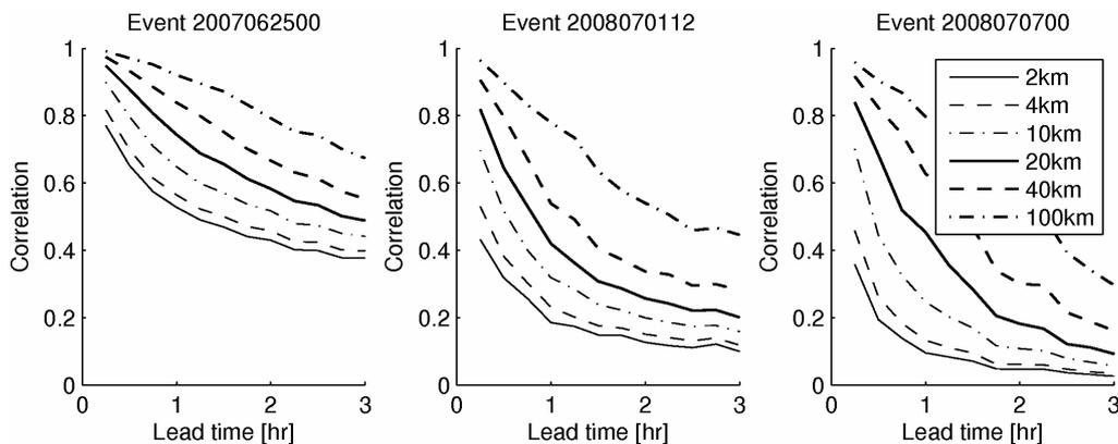
Figure 2 – Skill in the rain rate forecasts against lead time for a precipitation threshold of 0.125 mm/h.
