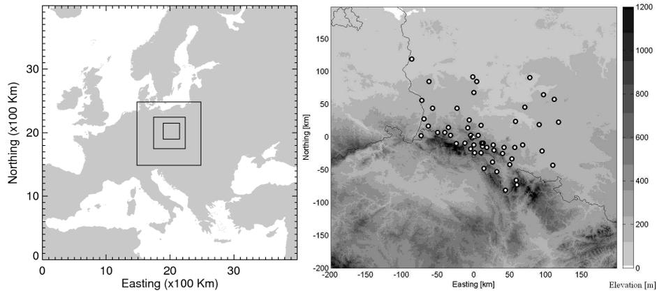
Figure 1. MM5 domains configurations (left, with four domains shown with solid boxes) and the weather radar coverage corresponding to domain 3 of MM5 (right, with triangle and circles representing the radar and rain gauge locations respectively).
