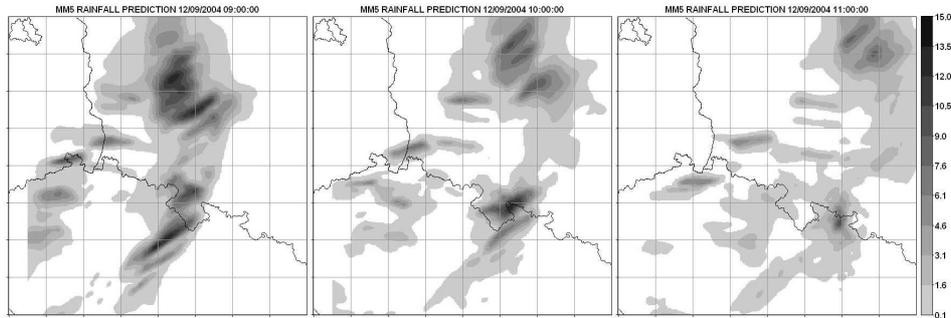
Figure 4. MM5 corrected using cross-correlation with radar at  $t=8$  hr (event: 2004/09/12).
